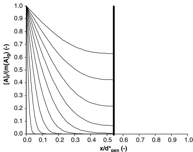
**Figure 7.** Concentration profiles for basecase with  $\delta = d_{\text{pen}}$  and parabolic velocity profile
