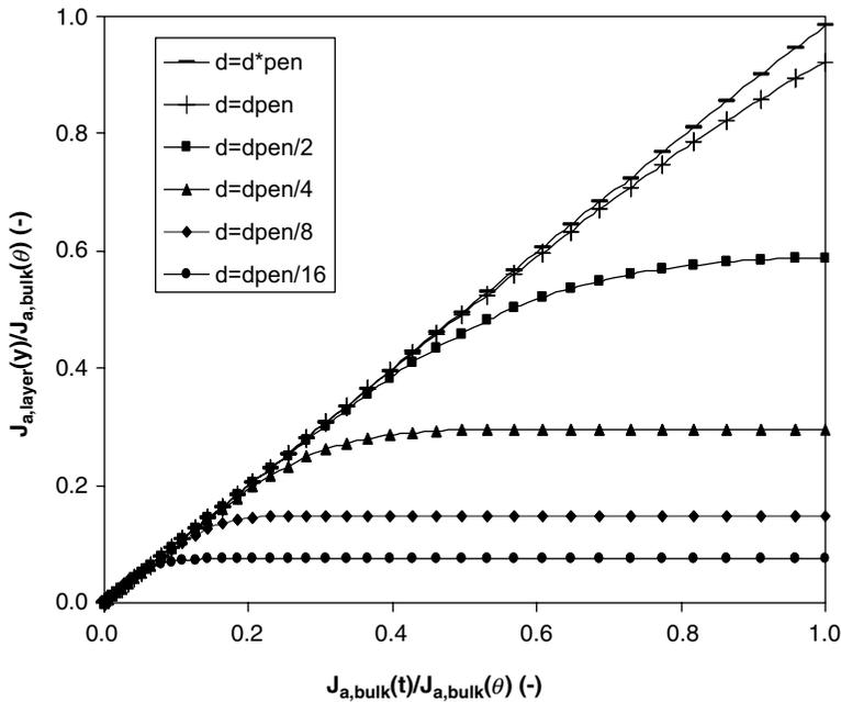
**Figure 8.** Cumulative (scaled) contribution of mass transfer flux with layer model versus bulk model at various layer thickness, parabolic velocity profile
