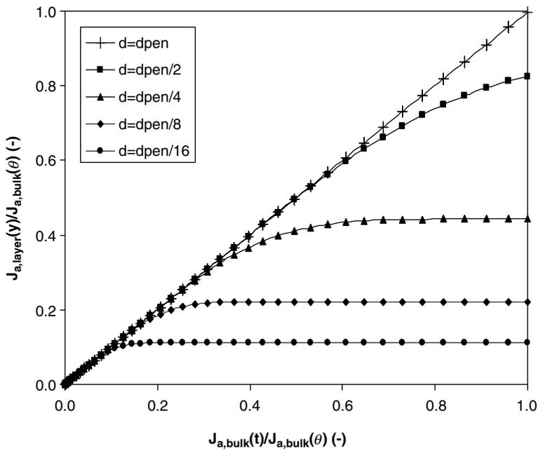
**Figure 6.** Cumulative (scaled) contribution of mass transfer flux with layer model versus bulk model at various layer thickness, plug flow velocity profile
