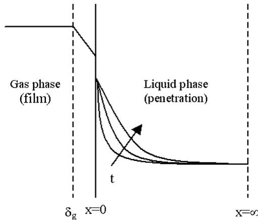
**Figure 1.** Penetration model for systems with liquid bulk
