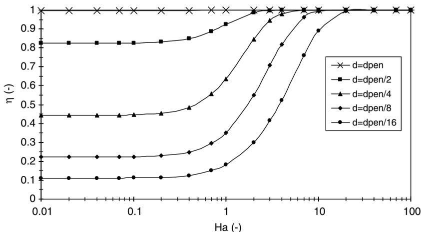
**Figure 9.** Mass transfer efficiency relative to system with liquid bulk. First order reaction, initially clean liquid, plug flow velocity profile
