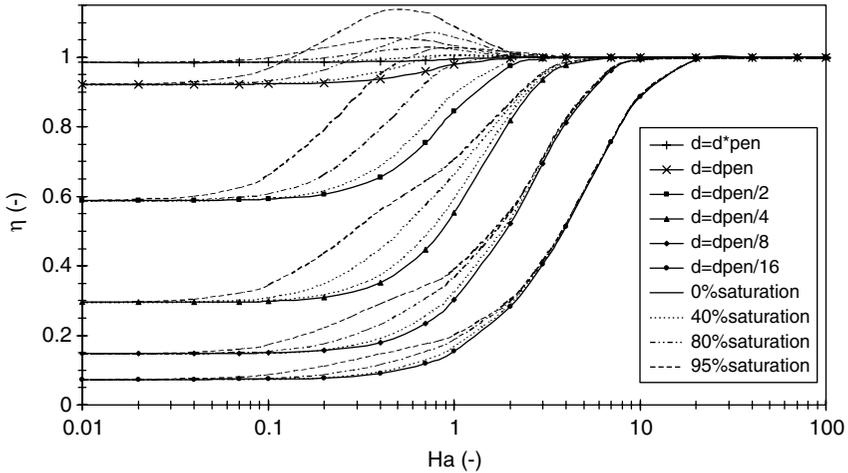
**Figure 12.** Mass transfer efficiency relative to system with liquid bulk. First order reaction, parabolic velocity profile
