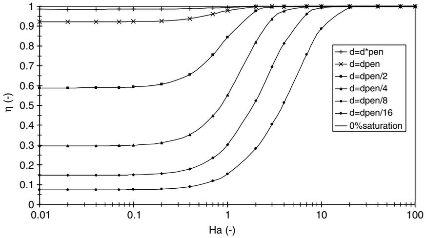
**Figure 11.** Mass transfer efficiency relative to system with liquid bulk. First order reaction, initially clean liquid, parabolic velocity profile
