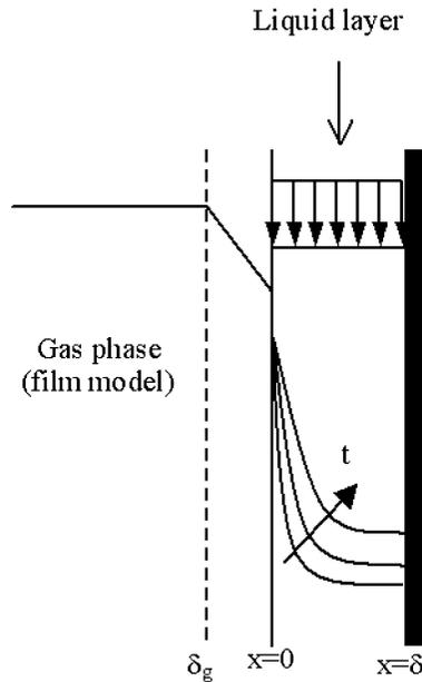
**Figure 2.** Penetration model for systems without liquid bulk
