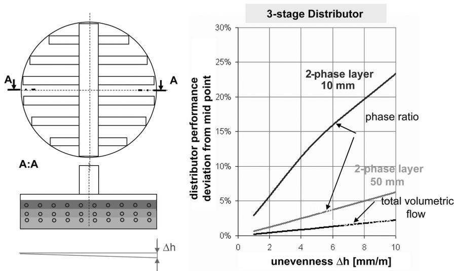
**Figure 2.** Three stage liquid distributor in two liquid phase applications
