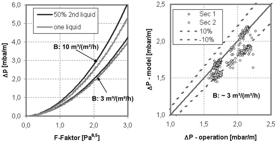
**Figure 3.** Pressure drop of three-phase distillation columns – model calculations for different liquid loads and a comparison to data points from a column in technical scale
