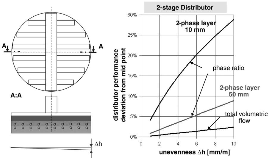
**Figure 1.** Distribution quality of a 2-stage distributor
