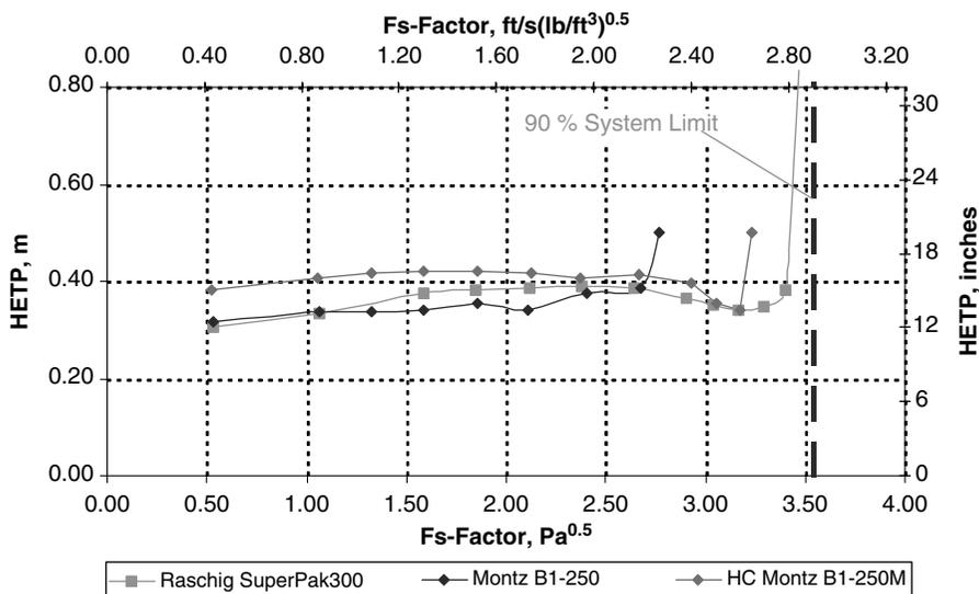
**Figure 4.** Mass transfer efficiency (HETP) comparison at total reflux. Raschig Super-Pak300 vs B1-250 and B1-250M at 0.33 bar, 0.43 m I.D. SRP column, 3.124 m bed, C<sub>6</sub>/C<sub>7</sub> system, high capacity distributor with drip tubes
