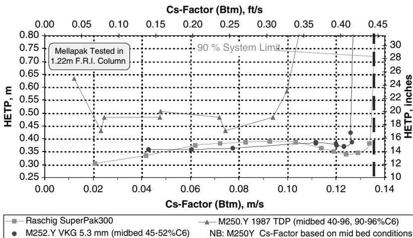
**Figure 6.** Mass transfer efficiency (HETP) comparison at total reflux. Raschig Super-Pak300 vs. F.R.I. tested M250Y and M252Y at 0.33 bar, 0.43 m I.D. SRP column, 1.22 m F.R.I. column,  $C_6/C_7$  system, high capacity liquid distributors
