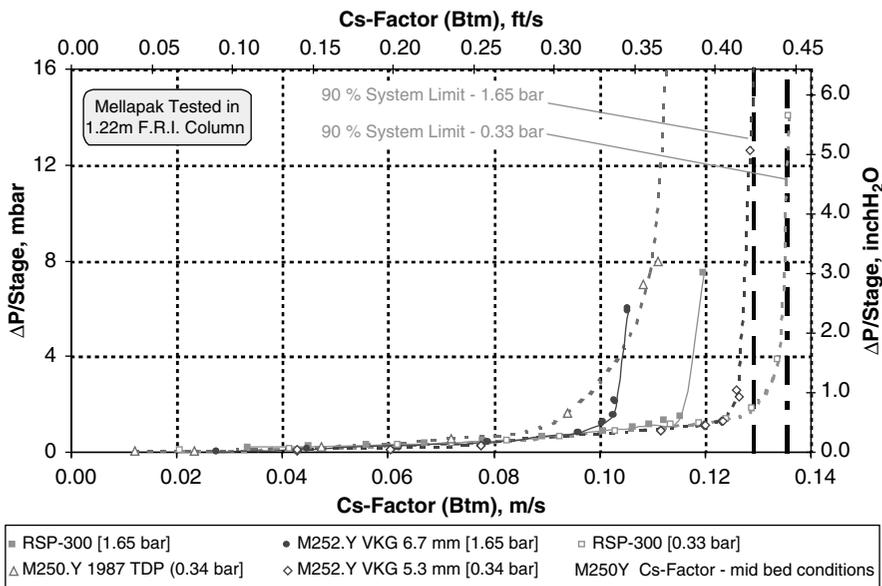
**Figure 10.** Pressure drop per theoretical stage comparison at total reflux. Raschig Super-Pak300 vs. F.R.I. tested M250Y and M252Y at 1.65 and 0.33 bar, 0.43 m I.D. SRP column, 1.22 m F.R.I. column, C<sub>6</sub>/C<sub>7</sub> system
