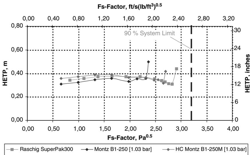
**Figure 3.** Mass transfer efficiency (HETP) comparison at total reflux. Raschig Super-Pak300 vs B1-250 and B1-250M at 1.65 bar, 0.43 m I.D. SRP column, 3.124 m bed, C<sub>6</sub>/C<sub>7</sub> system, high capacity distributor with drip tubes
