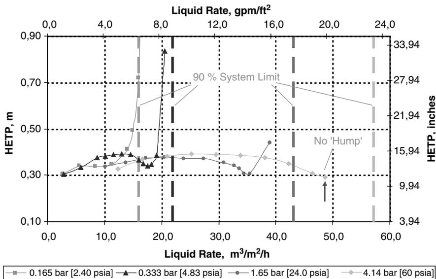
**Figure 2.** Effect of liquid rate and operating pressure on Raschig Super-Pak 300 HETP at total reflux. 0.43 m I.D. SRP column, 3.124 m bed, C<sub>6</sub>/C<sub>7</sub> system, high capacity distributor with drip tubes
