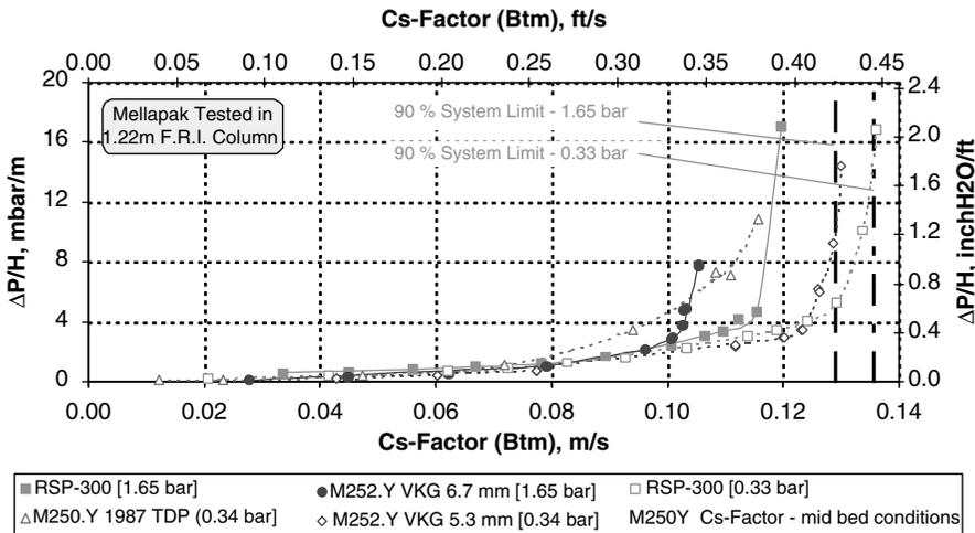
**Figure 8.** Pressure drop ( $\Delta P/H$ ) comparison at total reflux. Raschig Super-Pak300 vs. F.R.I. tested M250Y and M252Y at 1.65 and 0.34 bar, 0.43m I.D. SRP column, 1.22m F.R.I. column,  $C_6/C_7$  system, high capacity liquid distributors
