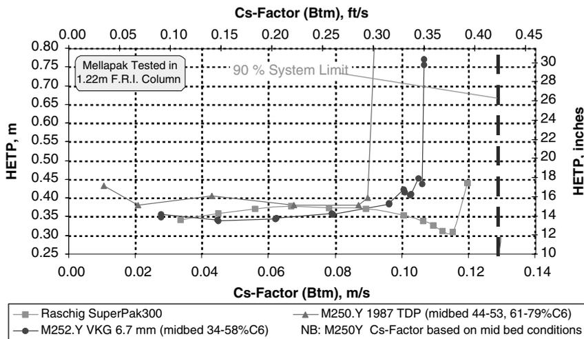
**Figure 5.** Mass transfer efficiency (HETP) comparison at total reflux. Raschig Super-Pak300 vs. F.R.I. tested M250Y and M252Y at 1.65 bar, 0.43 m I.D. SRP column, 1.22 m F.R.I. column,  $C_6/C_7$  system, high capacity liquid distributors
