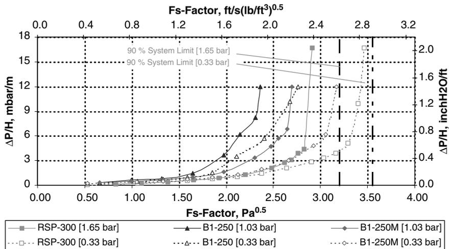
**Figure 7.** Pressure drop comparison at total reflux. Raschig Super-Pak300 vs. B1-250 and B1-250M at 1.65 and 0.33 bar, 0.43m I.D. SRP column, 3.124m bed,  $C_6/C_7$  system, high capacity distributor with drip tubes
