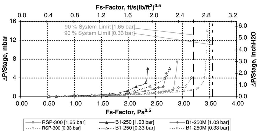
**Figure 9.** Pressure drop per theoretical stage comparison at total reflux. Raschig Super-Pak300 vs. B1-250 and B1-250M at 1.65 and 0.33 bar, 0.43m I.D. SRP column, 3.124m bed,  $C_6/C_7$  system
