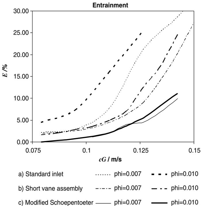
**Figure 3.** Air water entrainment  $E$  obtained in the simulator
