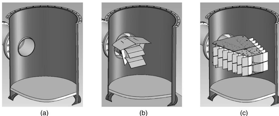
**Figure 1.** Inlet systems as installed in the 1 m diameter air/water simulator
