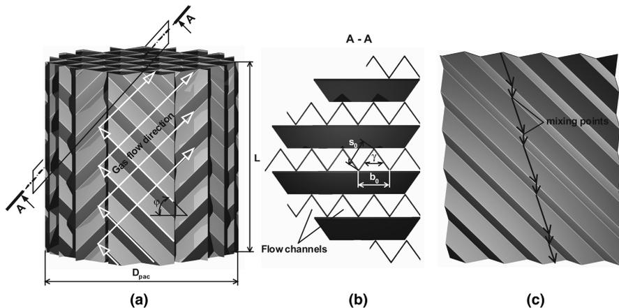
**Figure 2.** Schematic of the gas flow through a packing layer (a), sectional view illustrating geometry of the flow channels (b) and liquid flow path over the corrugated sheet surface (c)
