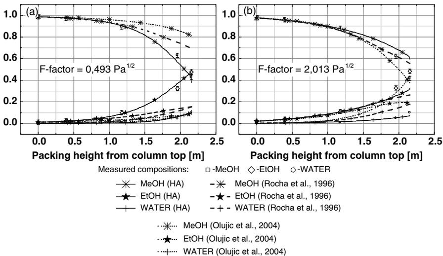
**Figure 6.** Predicted versus measured composition profiles (MeOH/EtOH/WATER) in a column with Montz-Pak B1-250 structured packing
