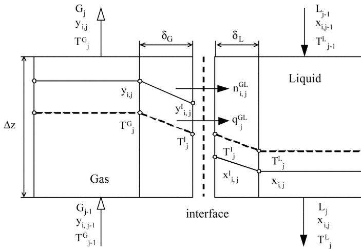
**Figure 1.** Schematic illustration of the two-film model
