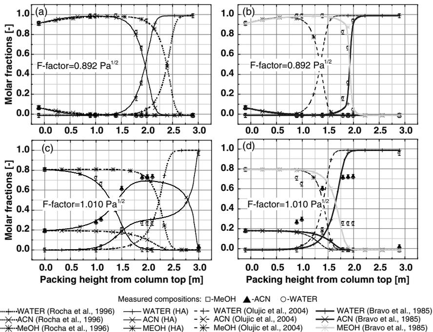
**Figure 5.** Predicted versus measured composition profiles (MeOH/ACN/WATER) in a column with Montz-Pak A3-500 structured packing
