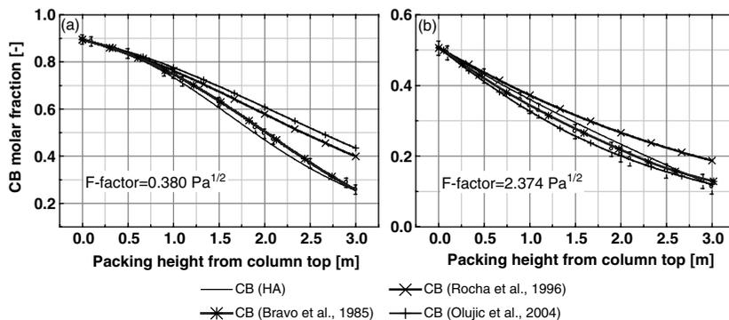
**Figure 4.** Predicted (lines) versus measured (circles) CB/EB composition profiles in a column with Montz-Pak A3-500 structured packing
