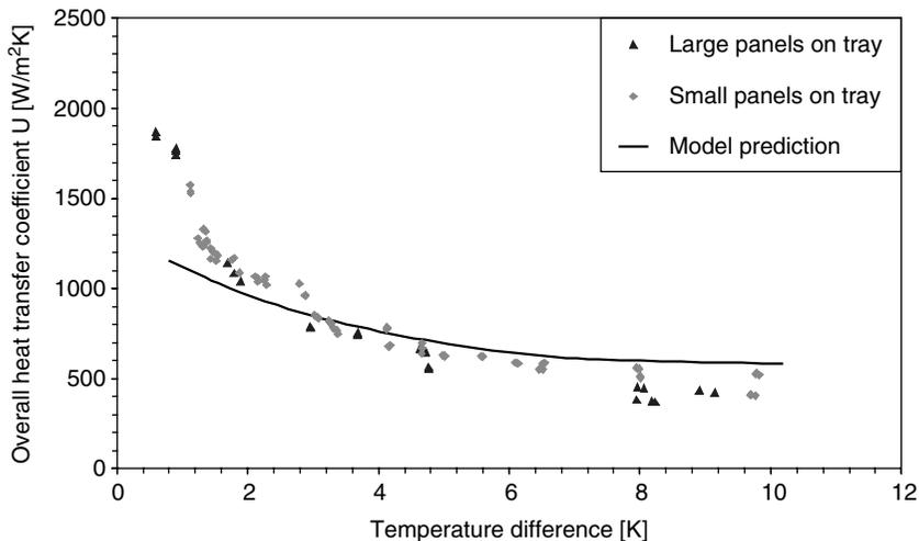
**Figure 3.** Overall heat transfer coefficient for heat transfer panels placed on active area of annular tray
