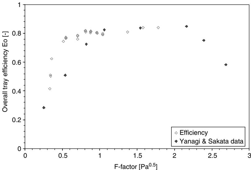
**Figure 4.** Overall tray efficiency of annular tray compared to conventional cross flow sieve tray tested by FRI
