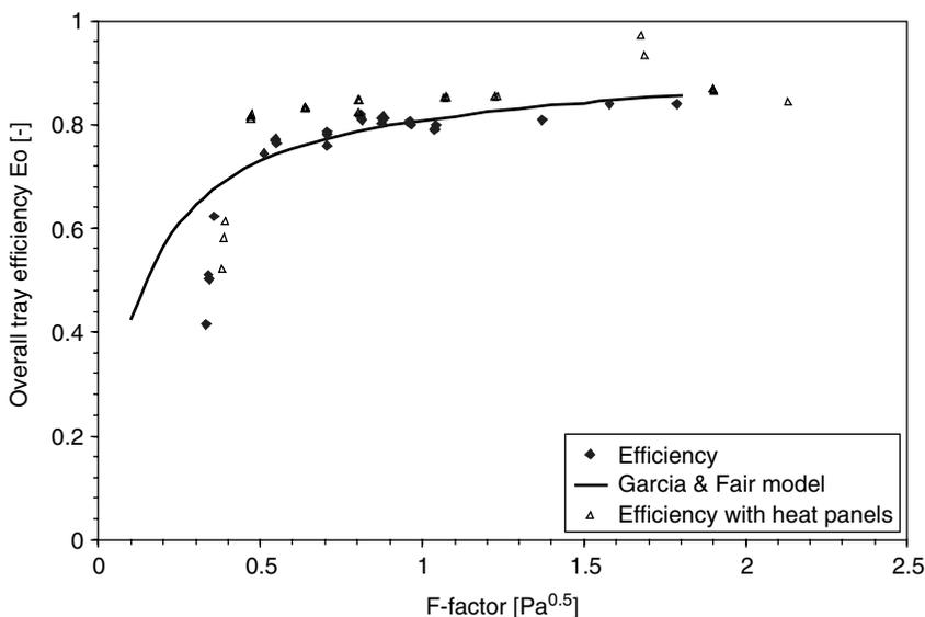
**Figure 5.** Overall tray efficiency as function of F-factor
