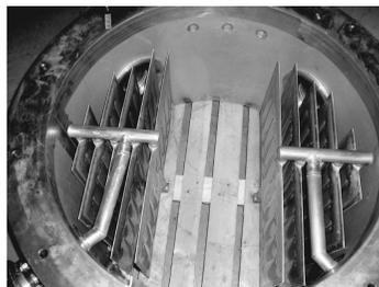
**Figure 2.** Placement of heat transfer panels in stripping section (a) and orientation of heat transfer panels in pilot plant (b)
