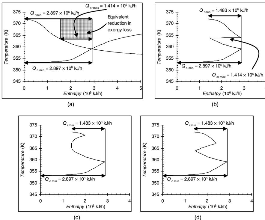
**Figure 3.** Active IRS curves for different way of incorporating side reboiler: (a) side reboiler targets; (b) withdrawing liquid and returning at the same location; (c) withdrawing 10 kmol/h of liquid and returning at different location; and (d) withdrawing 36 kmol/h of liquid and returning at different location
