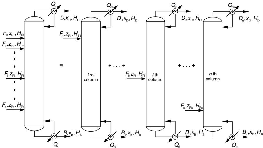
**Figure 1.** Decomposition of complex distillation column with  $n$  feeds into  $n$  single-feed distillation columns
