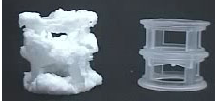
Figure 1: Crystallization fouling on the surface of a single Pall-Ring (left side) / clean Pall-Ring (right side)
