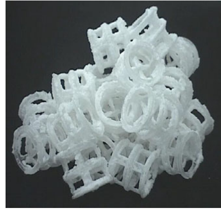
Figure 2: Crystallization fouling on a random packing
