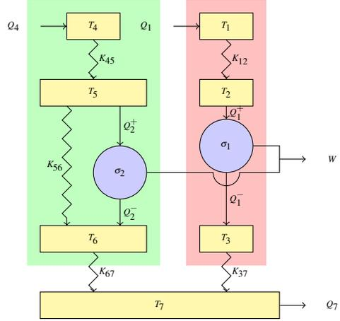
Figure 3: Diagram corresponding to a thermodynamically consistent model of a flex-fuel generation facility. The left path corresponds plant performance when coal-fired, the right path corresponds to the more efficient natural gas generating capability of the plant. For details, see [5].
