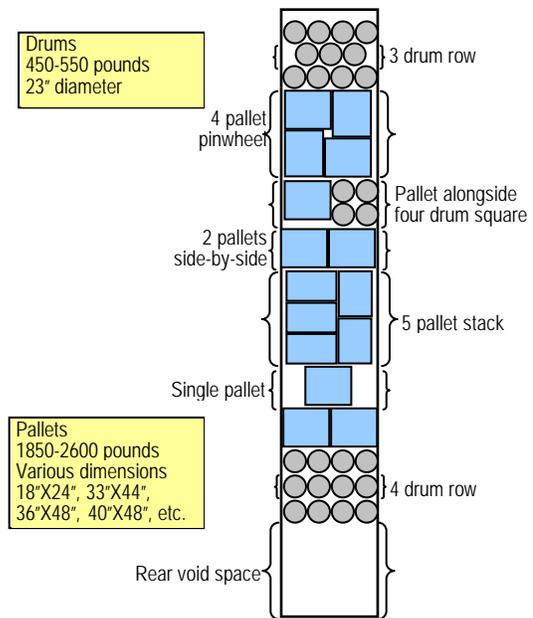
Figure 7. Standard semi-trailer packages
