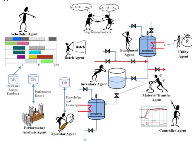
*Figure 9. Agent-based real-time batch management system*
