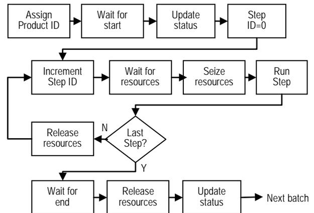
Figure 5. Generic simulation logic
