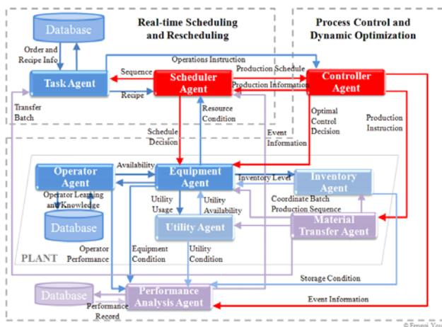
Figure 10. Expected architecture of the MAS
