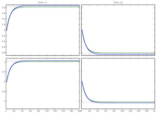
Fig. 7. Comparison of the estimated model with the true system (green - model, blue - true system).
