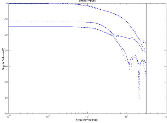
Fig. 4. Comparison of the singular values - estimated model (dash-dotted) with the true system (solid).
