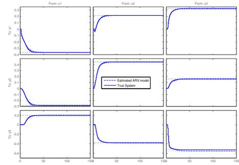
Fig. 2. Comparison of the estimated model (dash-dotted) and actual (solid) step responses from the experiment data.
