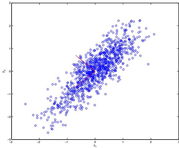
Fig. 5. Open loop excitation shown in the output space (red straight lines denote the directions of the two column vectors in  $V$ ).
