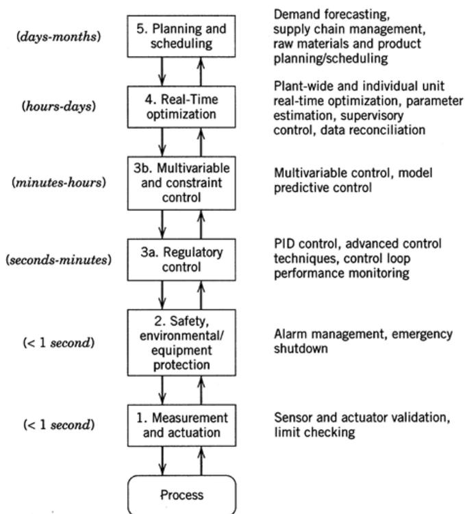
Figure 4. The five levels of process control and optimization in manufacturing. Time scales are shown for each level (Seborg et al., 2010)
