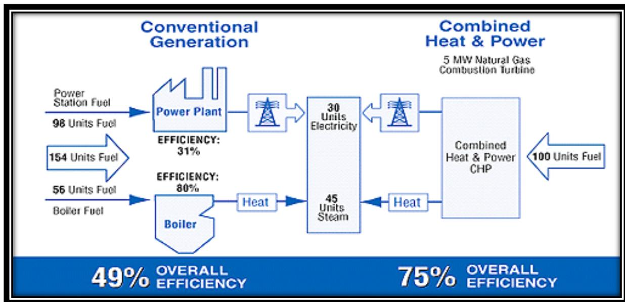
Figure 2 Comparison of energy flows for conventional generation vs. combined heat and power (cogeneration), Source: EPA.
