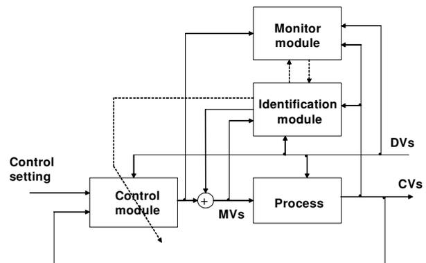
Figure 1. Block diagram of the semi-automatic MPC
