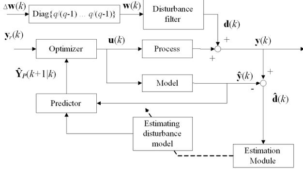
Figure 7. MPC controller with the adaptive disturbance model
