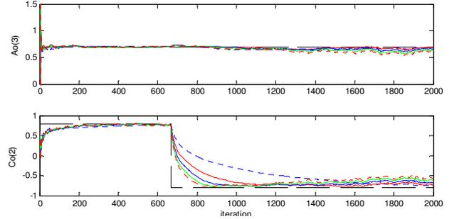
Figure 8. Parameter plots in the simulation study. Parameter  $c_2$  jumped at sample 660. The blue dashed lines are the parameters estimated using traditional PLR, other lines are the parameters estimated using the new MIPLR with increasing iteration number
