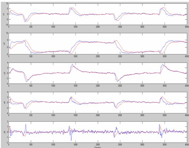
Figure 11. MVs of the old MPC (red lines) and that of the new MPC (blue lines). MVs of the new MPC moves ahead of that of the old MPC
