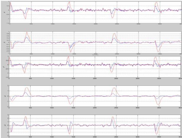
Figure 10. CVs of the old MPC (red lines) and that of the new MPC (blue lines). CV peaks can be reduced 50%.
