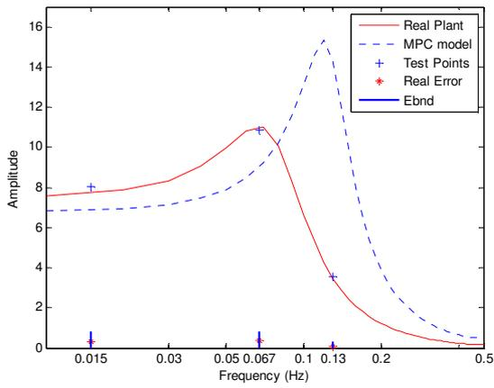
Figure 13. Frequency responses of the process (red line) and that of the MPC model (blue line)
