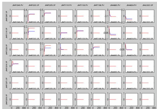
Figure 6. The old (blue) and the new (red) models for a section of the MV/CVs
