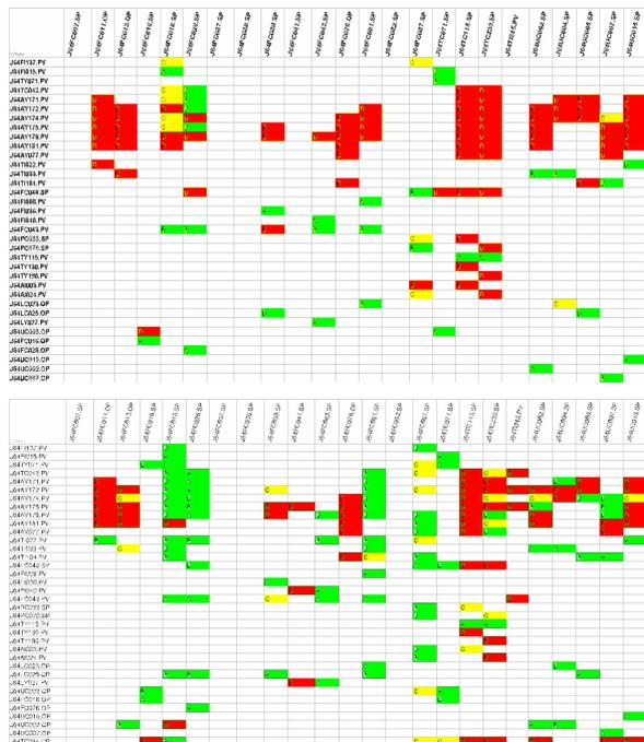
Figure 5. (Upper) Model qualities after day 1 of step testing and (Lower) after 4 days of step testing. Red – D quality models, Yellow – C quality and Green – A/B quality models. Blank entries in the matrixes means that there is no model expected
