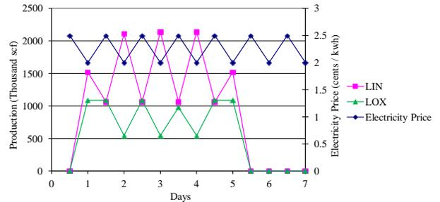
Figure 2. Production rate vs. electricity prices for plant 1
