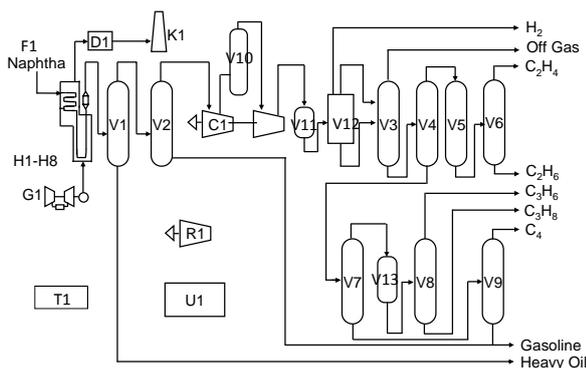
Fig. 3 Process flow diagram for ethylene plant (Higuchi et al., 2010)
