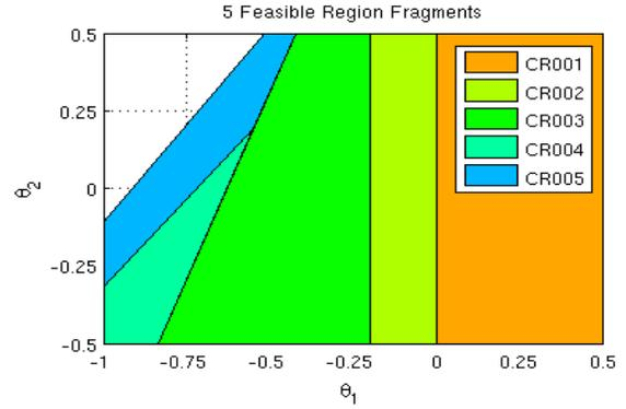
Figure 2. Critical Regions of Example 1 with Two-Stage Method
