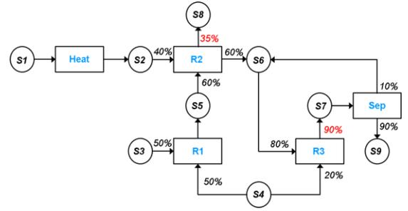
Figure 4. STN-Representation of Example 2 with Nominal Conversion Rates
