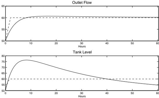
Figure 3. Step responses to an inlet flow change from 50% to 60% for the optimal controller, (10), (solid) and the robust controller, (19), (dashed).
