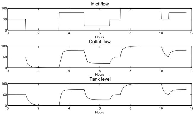
Figure 2. Simulation of closed loop robust MPC with a sampling period of one minute, a prediction horizon of 60 minutes and  $k_v = \frac{1}{10}$ .
