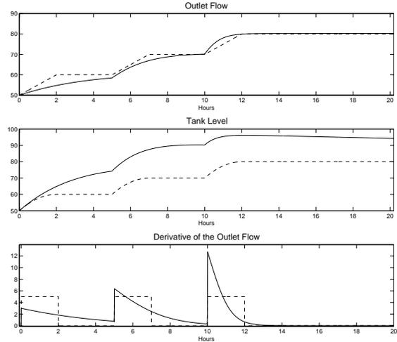
Figure 4. The optimal controller (solid) and the robust controller (dashed) for inlet flow steps of size 10% every five hours and  $k_v = 1$ .
