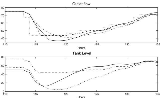
Figure 5. Outlet and tank level for the optimal MPC<sup>2</sup> (solid), robust (dashed) and optimal (dash-dotted) controllers.
