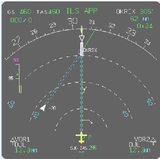
Figure 1: Merge behind application on CDTI in real time experiments.
