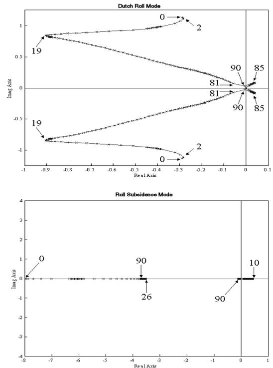
Fig. 4. Dutch Roll, Spiral and Roll Subsidence Mode Movement
