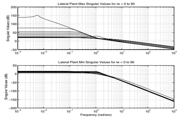
Fig. 6. Lateral Plant Singular Values for  $i_w = 0^\circ$  to  $90^\circ$  Finally, examining the direction vectors corresponding to the maximum singular value will be useful in determining the coupling between the inputs and outputs at various points of the conversion.
