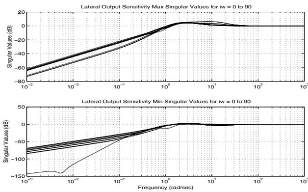
Fig. 10. Lateral Sensitivity Singular Values at Plant Output
