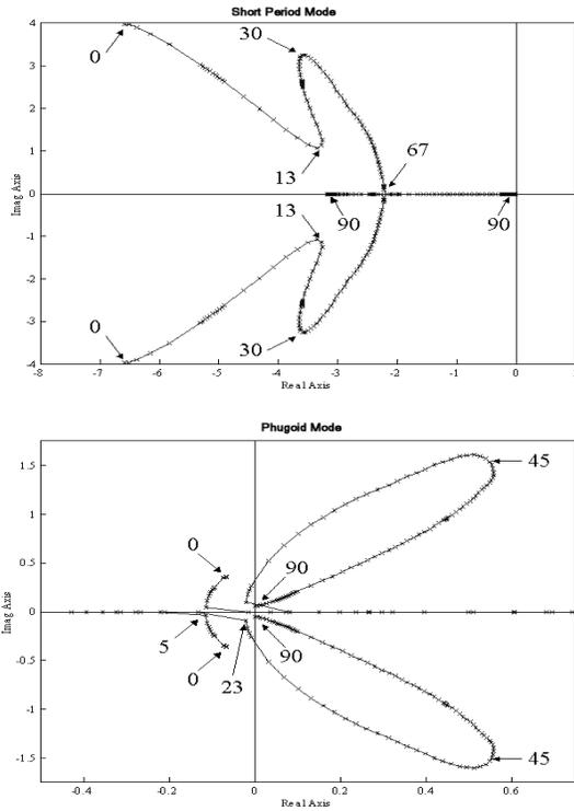
Fig. 3. Short Period and Phugoid Mode Movement During Conversion
