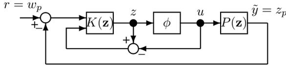
Fig. 6. An example of anti-windup control system.
