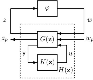
Fig. 1. Feedback control system with dead-zone nonlinearities.
