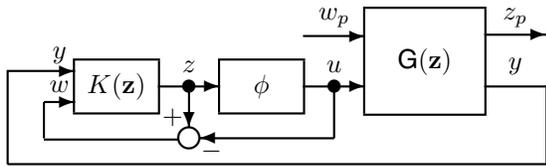
Fig. 5. Anti-windup control system.
