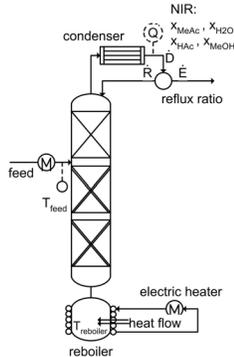
Fig. 3. Scheme of the semibatch reactive distillation column.
