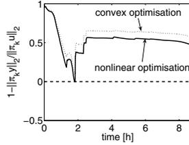
Fig. 6. Unfalsification constraints over time, model is invalidated below the dashed line.
