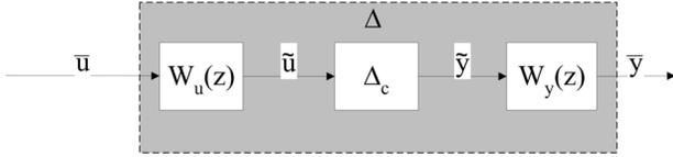
Fig. 2. Internal structure of  $\Delta$
