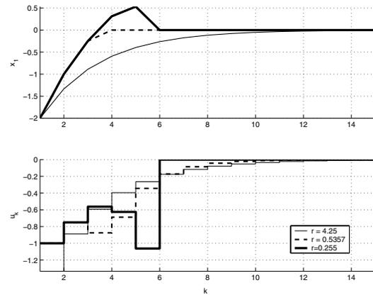
Fig. 5. Response of the system in example 4.1 and the corresponding control action as the tuning “dial” changes parameter  $r$  from 0.01 to 4.5.
