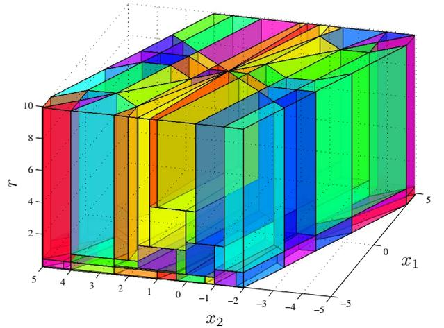
Fig. 2. Explicit solution to the MPC problem in example 4.1 with control weight as a parameter (154 critical regions).
