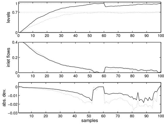
Fig. 1. Liquid levels, inlet flows and absolute deviation (from the exact MMMPC) of the proposed strategy (tank 1 solid plot, tank 2 dotted plot).
