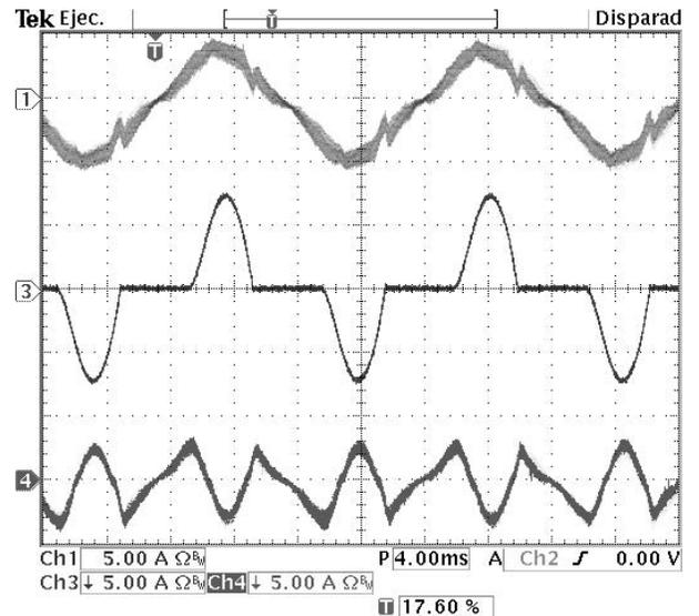
Fig. 4. (from top to bottom) compensated current  $i_S(t)$ , current load  $i_0(t)$ , and injected current  $i(t)$ .
