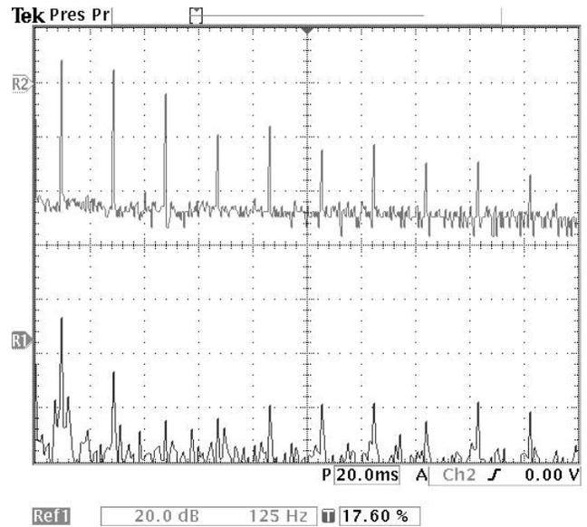
Fig. 7. Spectra of (top) the load current  $i_0$ , and (bottom) the compensated current  $i_S$ .
