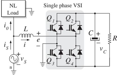
Fig. 1. Single phase full-bridge shunt active filter.
