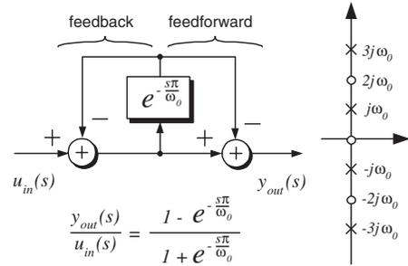
Fig. 2. Block diagram and poles location of the proposed negative feedback repetitive compensator with feedforward path.
