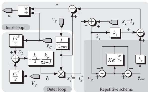
Fig. 3. Block diagram of the proposed repetitive-based controller.
