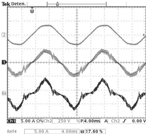
Fig. 5. (from top to bottom) Source voltage  $v_S(t)$ , source current  $i_S(t)$  with harmonic compensation, and source current  $i_S(t)$  without harmonic compensation.
