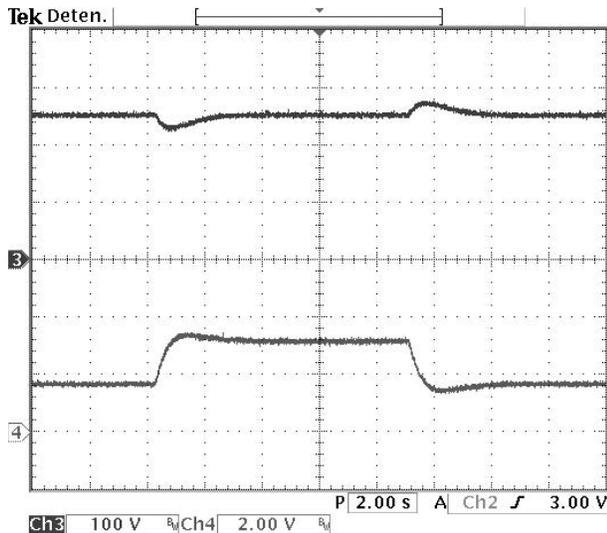
Fig. 6. (top) Capacitor voltage  $v_C(t)$ , and (bottom) scaled apparent conductance  $\delta(t) = v_{S,RMS}^2 \eta(t)$  observed by the source.
