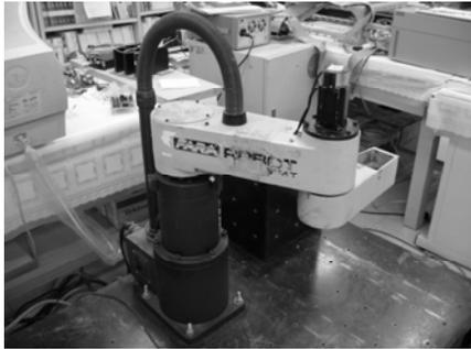
Fig. 11. SCARA type robot system
