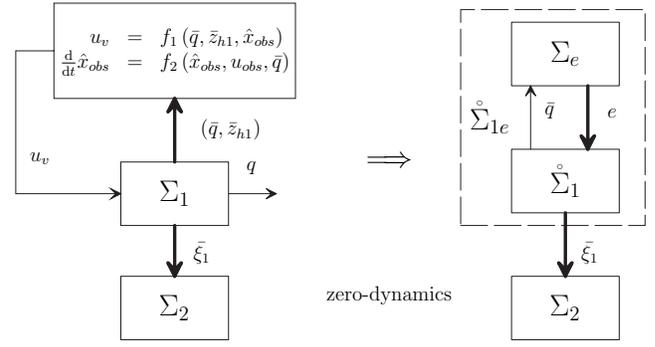
Fig. 2. The structure of the plant with the dynamic controller and the corresponding PH systems.
