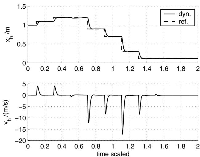
Fig. 5. Piston position ( $x_h$ ) and velocity ( $v_h$ ) responses with dynamic controller over a large position range.
