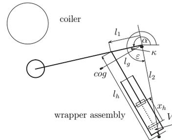
Fig. 3. The wrapper assembly with center of gravity (cog).
