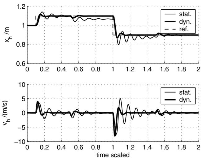
Fig. 4. Piston position ( $x_h$ ) and velocity ( $v_h$ ) responses with static and dynamic controller.
