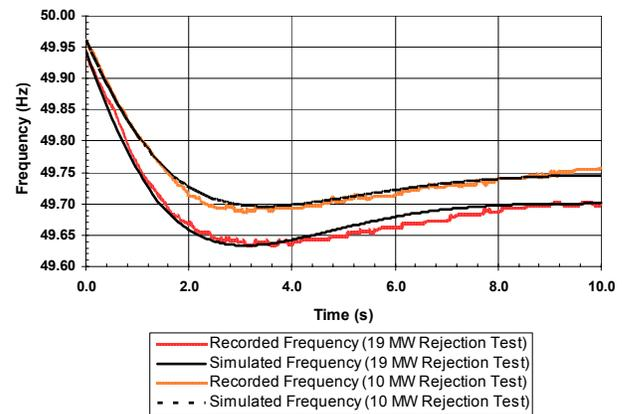
Fig. 7. Measured and simulated system frequency for the 10 MW and 19 MW rejection tests.
