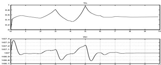
Fig. 6. Engine dynamic:  $T_h$  control input and angular rotor velocity  $w_r$ .
