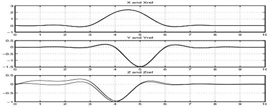
Fig. 4. Trajectory followed over desired path in X, Y and Z.
