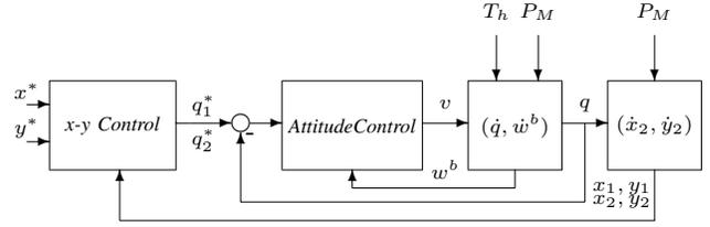
Fig. 2. lateral/longitudinal/attitude control structure.
