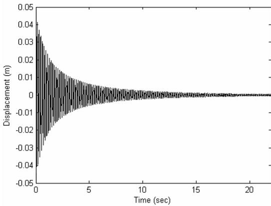
Fig.6, Free response of the beam for 0.04 m tip point displacement.
