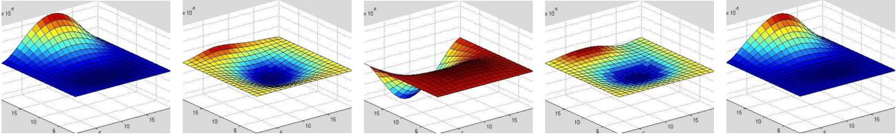
Fig. 1. Simulation of the uncontrolled Mindlin plate. The system is clamped except along the  $x = L_x$  side.
