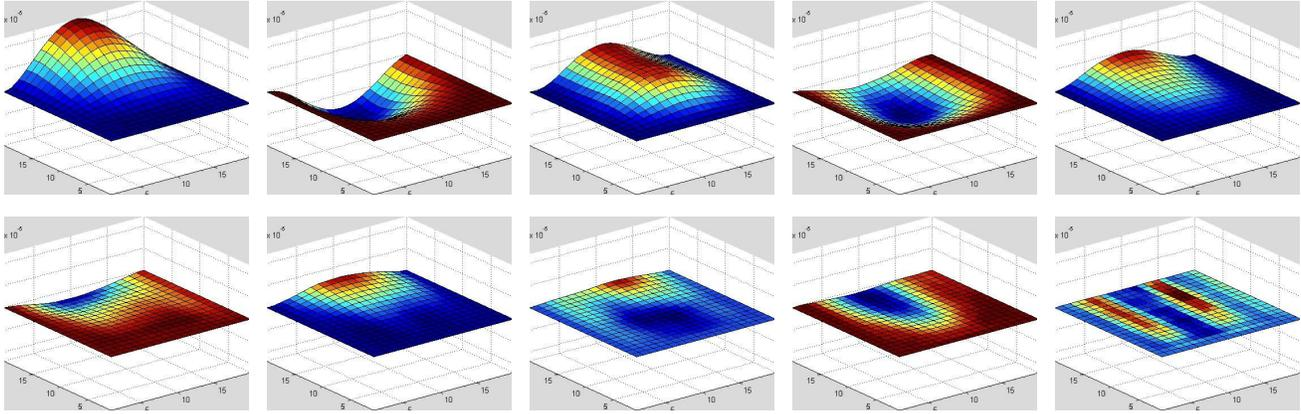
Fig. 2. Simulation of the boundary controller by damping injection. The controller is interconnected to the system along the  $x = L_x$  side, while the plate is clamped on the others.
