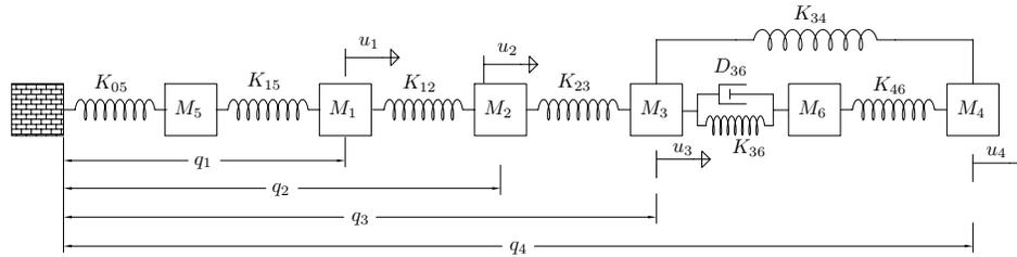
Fig. 3. The mechanical system considered in Example 1.
