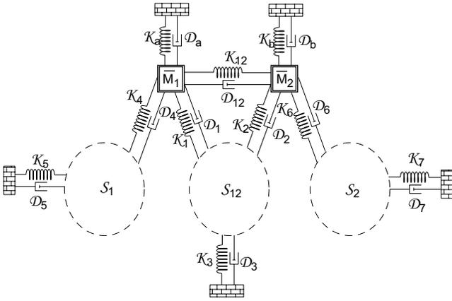
Fig. 2. Decomposition of the given system. For space reasons springs and dampers are depicted in different directions, but the reader should imagine all the motions as horizontal.
