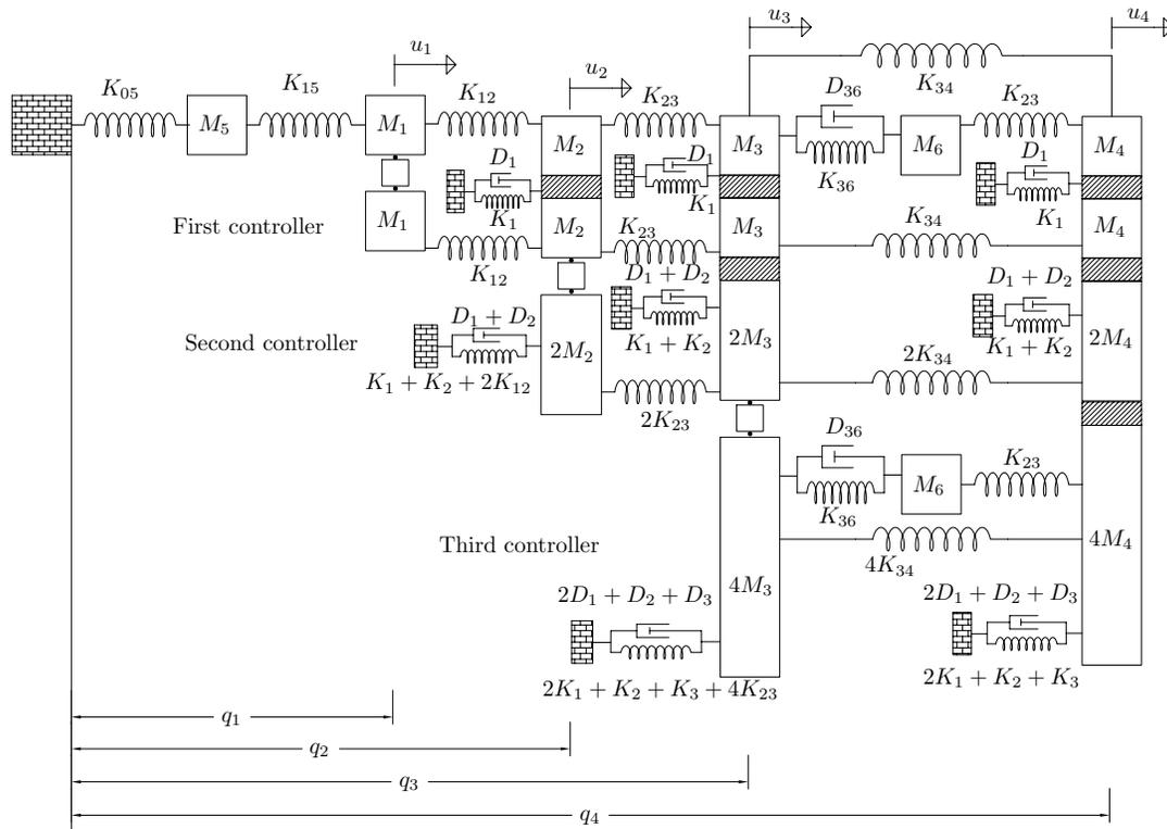
Fig. 4. The overall mechanical system considered in Example 1.
