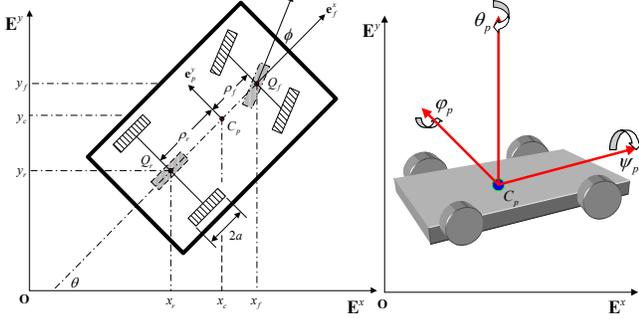
Fig. 1. The configuration of the car-like mobile robot.
