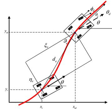
Fig. 3. Current vs. desired configuration of the mobile robot
