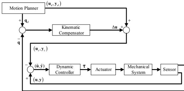
Fig. 2. The block diagram of hierarchical control design.
