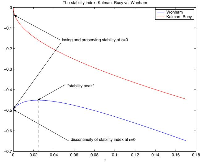
Fig. 1. Different behavior of the stability exponent for linear and nonlinear filter
