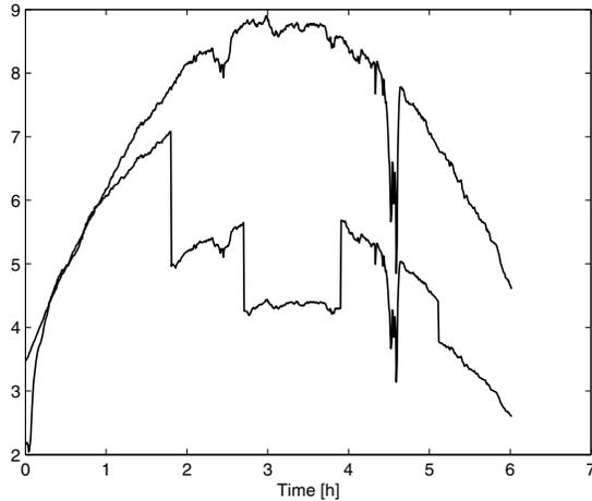
Fig. 8. Closed loop with RHC having  $T = 180$  s. Radiation (disturbance – above) ( $\times 1 \times 10^{-2}$ ) [ $W/m^2$ ] and oil flow (manipulated variable – below) ( $\times 1 \times 10^4$ ) l/s.
