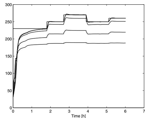
Fig. 7. Closed loop with RHC having  $T = 180$  s. Outlet oil temperature and reference and temperature estimates at the collocation points.
