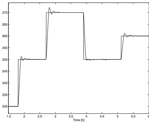
Fig. 4. Closed loop with RHC having  $T = 60$  s. Outlet oil temperature and reference. Detail
