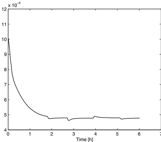
Fig. 9. Closed loop with RHC having  $T = 180$  s. Mirror efficiency estimate,  $\hat{\alpha}$ .
