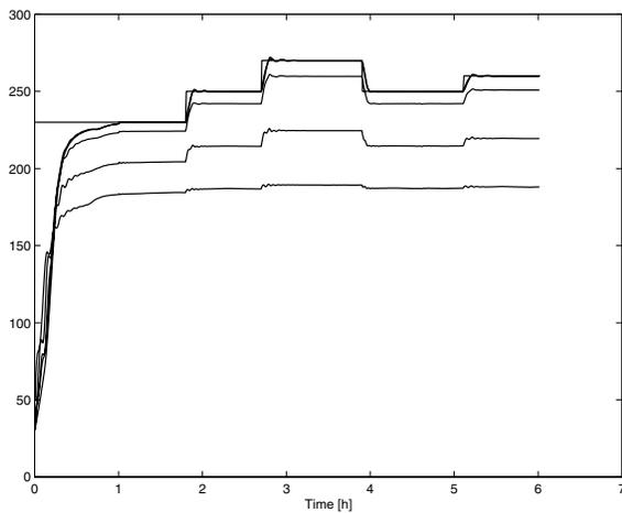
Fig. 3. Closed loop with RHC having  $T = 60$  s. Outlet oil temperature and reference and temperature estimates at the collocation points.
