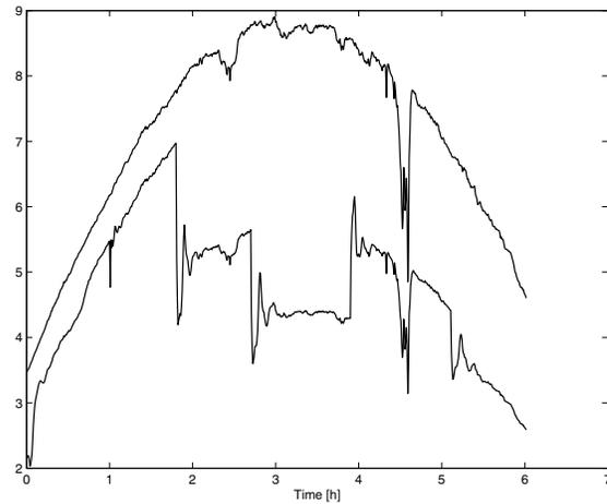
Fig. 5. Closed loop with RHC having  $T = 60$  s. Radiation (disturbance - above) ( $\times 1 \times 10^{-2}$ ) [ $W/m^2$ ] and oil flow (manipulated variable - below) ( $\times 1 \times 10^4$ )  $l/s$ .
