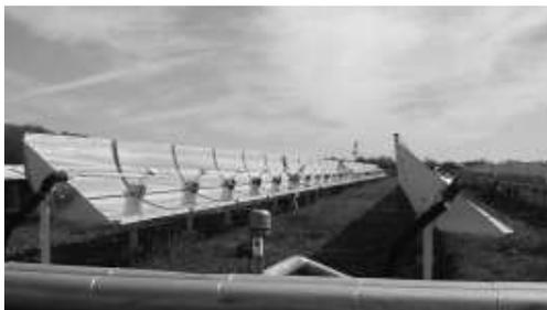
Fig. 1. A view of one collector loop with the pipe in the focus of the concentrating mirrors.
