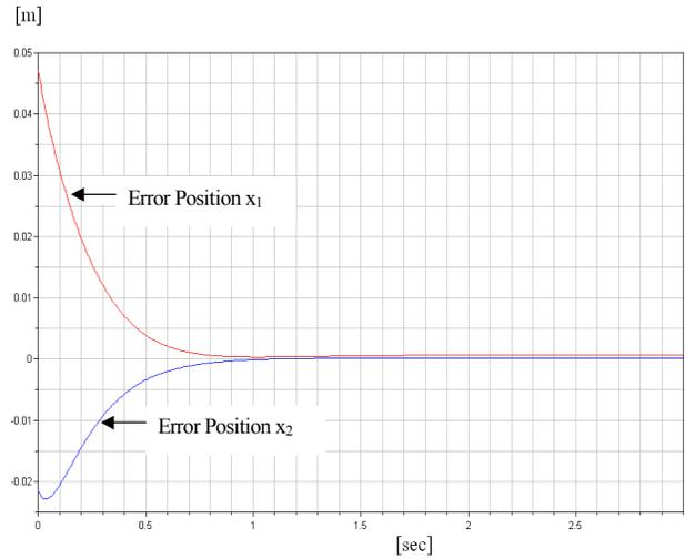
Fig. 3. End-effector position error
