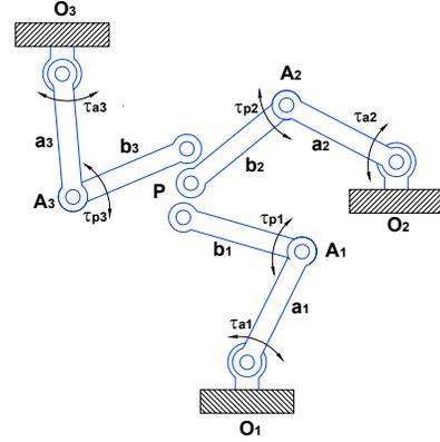
Fig. 2. Parallel robot in its open-chain form
