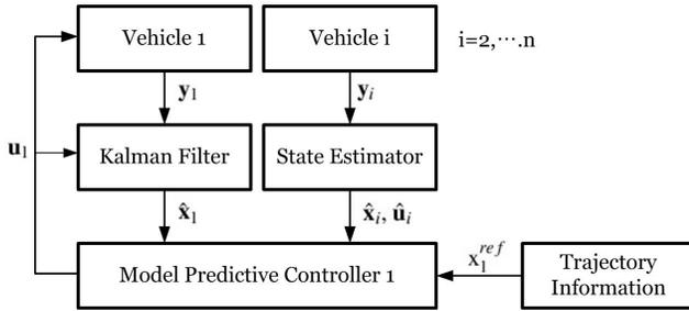
Fig. 2. Control block diagram at Vehicle 1
