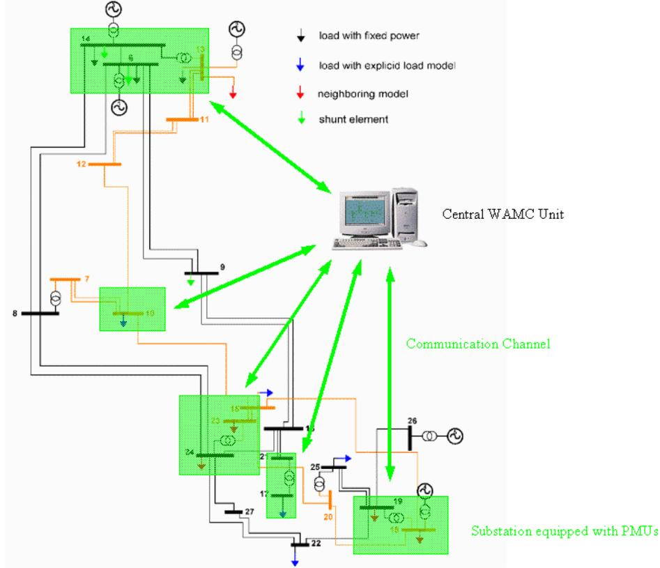
Fig. 2. Setup of wide area platform based on synchronized phasor measurements.
