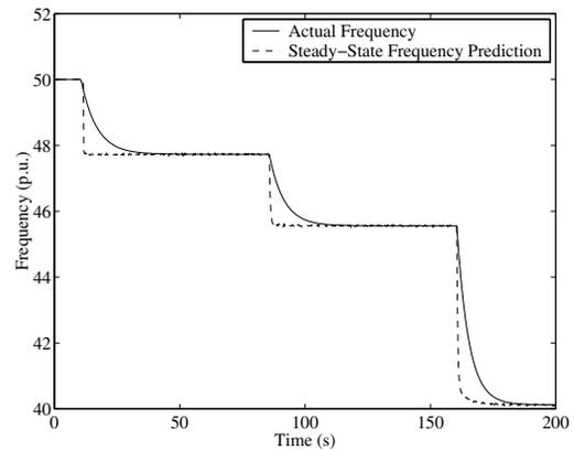
Fig. 5. Frequency response and steady-state frequency prediction in the simulation with disconnection of the three units G3, G4 and G5 at 10.1 s, 85.2 s and 160 s, respectively.
