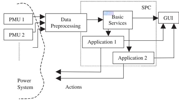
Fig. 3. Functional architecture of wide area measurement platform based on synchronized phasor measurements.
