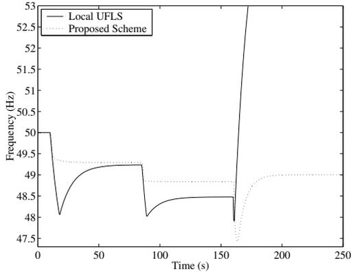
Fig. 8. Comparison of frequency response with local UFLS and the proposed scheme.
