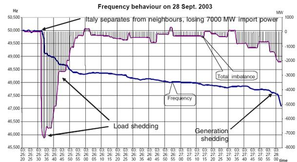
Fig. 1. The frequency and estimated power imbalance during the Italian grid collapse of 2003 [3].
