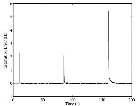
Fig. 6. Steady-state frequency prediction error following the three unit trippings.
