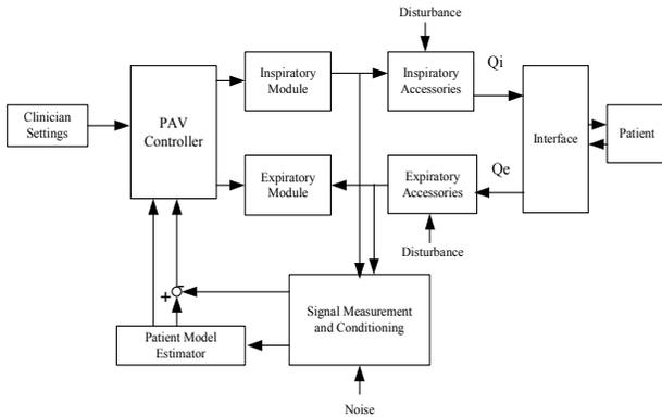
Fig. 2 PAV patient-ventilator modular block diagram.
