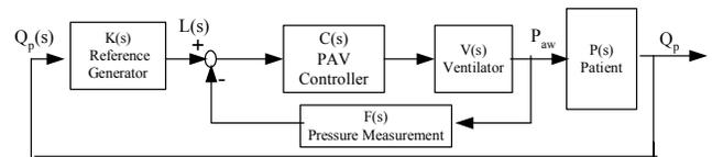
Fig. 3 Simplified PAV system for inspiration phase.
