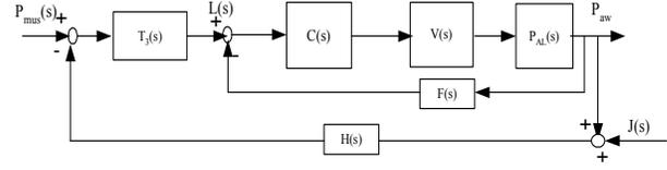
Fig. 5 Conceptual closed-loop block diagram including patient airway-lung model,  $P_{AL}(s)$ , physiologic control dynamics,  $H(s)$ , and physiologic inputs,  $J(s)$ .
