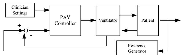
Fig.1 PAV conceptual framework demonstrating patient-generated tracking reference.
