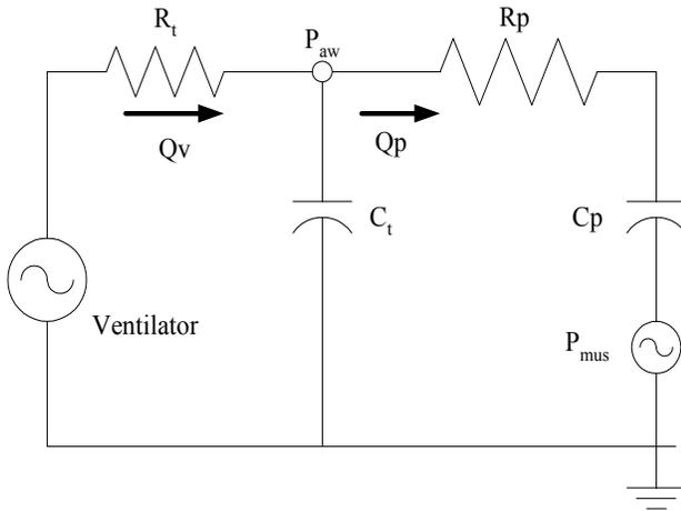
Fig. 4 Simplified analog model for patient circuit and lung.
