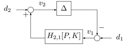
Fig. 5. Robust feedback loop block diagram
