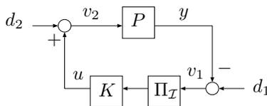
Fig. 4. Feedback loop with measurement data rate constraint
