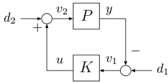
Fig. 1. The standard feedback loop block diagram
