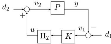
Fig. 3. Feedback loop with control data rate constraint
