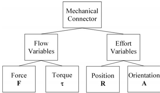
Fig. 1. Mechanical Connector Scheme
