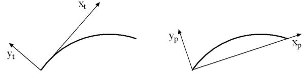
Fig. 3. Tangent (left) and pinned (right) reference systems
