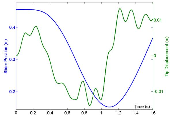
Fig. 7. Slider block position and tip transverse displacement of the connecting rod
