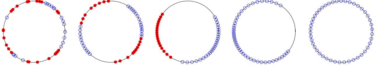
Fig. 1. The agree-and-pursue control and communication law in Section II-C with  $N = 45$ ,  $r = 2\pi/40$ , and  $k_{\text{prop}} = 1/4$ . Disks and circles correspond to agents moving counterclockwise and clockwise, respectively. The initial positions and the initial directions of motion are randomly generated. The five pictures depict the network state at times 0, 12, 37, 100, 400.
