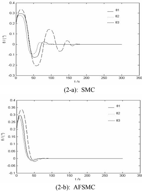
Fig. 2. Attitude angles in the case of no external disturbance
