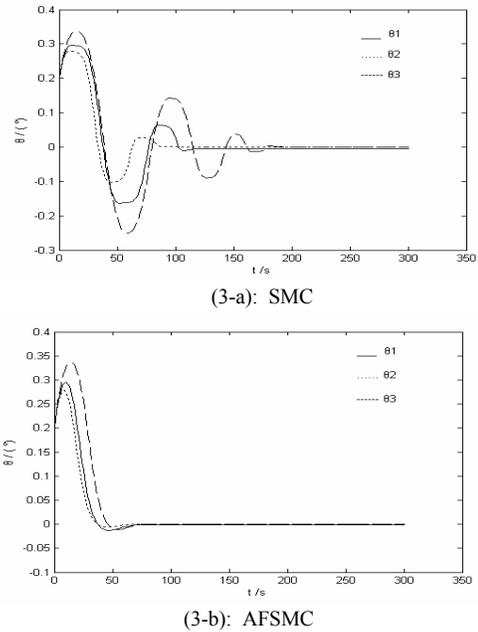
Fig. 3. Attitude angles in the case of the external disturbance
