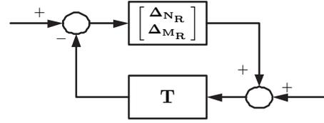
Fig. 2. Standard form for closed-loop system.
