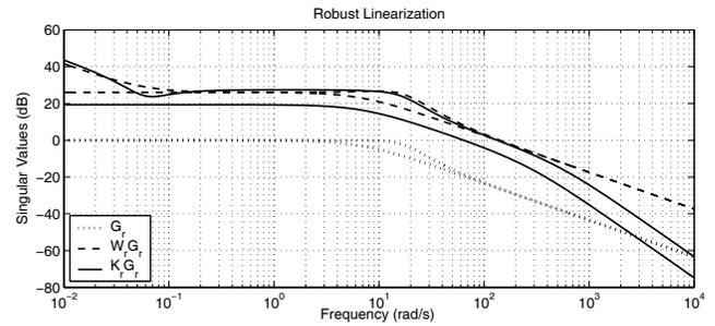
Fig. 5. Singular value plots of  $G_r$ ,  $W_r G_r$  and  $K_r G_r$ .
