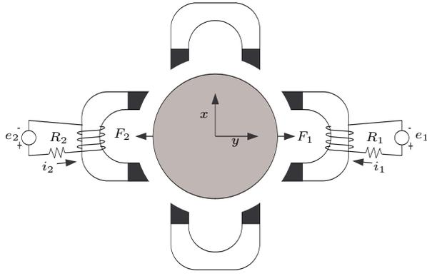
Fig. 3. Top view of a planar rotor disk magnetic bearing system [8].
