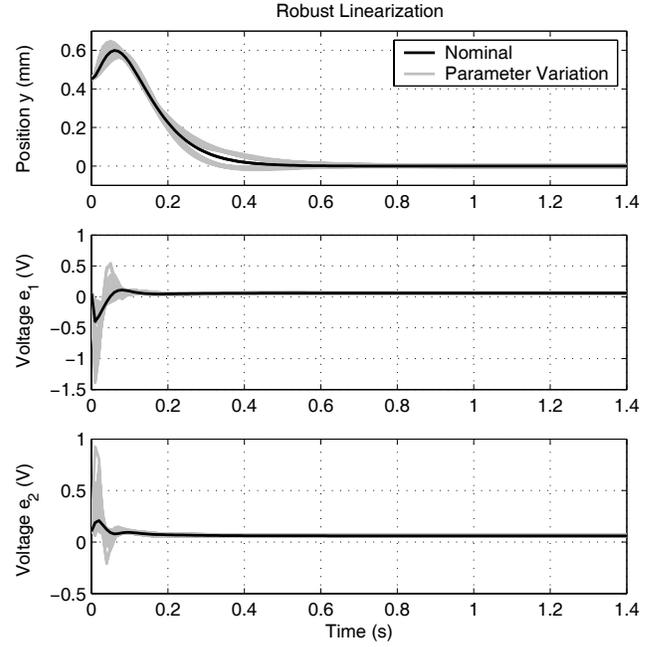
Fig. 8. Position  $y$  and voltages  $e_1$  and  $e_2$  for the robust linearization.
