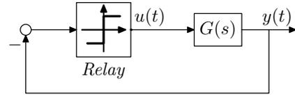
Fig. 2. Closed loop system composed of a SPR linear unit and a time-variant relay.
