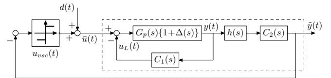
Fig. 3. VSC control scheme with exact differentiations.
