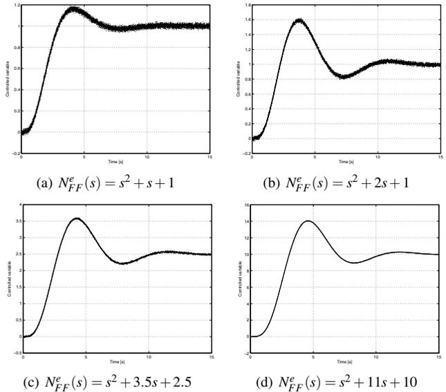
Fig. 3. Controlled variable estimated from the output base functions.
