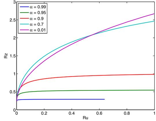
Fig. 1. Output variance,  $R_z$ , versus input variance,  $R_u$ , for different values of  $\alpha$ . The curves are generated by varying  $S$ . In all cases the lowest output variance is obtained by turning the controller off (i.e.  $S \rightarrow \infty$ ).
