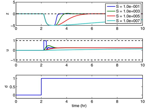
(b) Closed-loop response of input constrained MPC.
