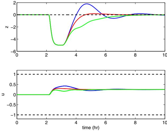
Fig. 5. The closed-loop response of the constrained MPC with  $(S, \alpha) = (10^5, 0.7)$  and a model corresponding to the gains  $K = 40$  (blue),  $K = 20$  (red), and  $K = 10$  (green). The plant has gain  $K = 20$ . This controller is robust to plant-model mismatch.
