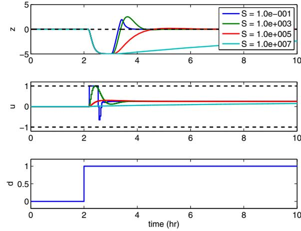
(b) Closed-loop response of input constrained MPC.
