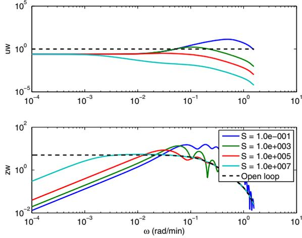
(a) Closed-loop frequency response analysis. Amplitude of  $u$  and  $z$ .
