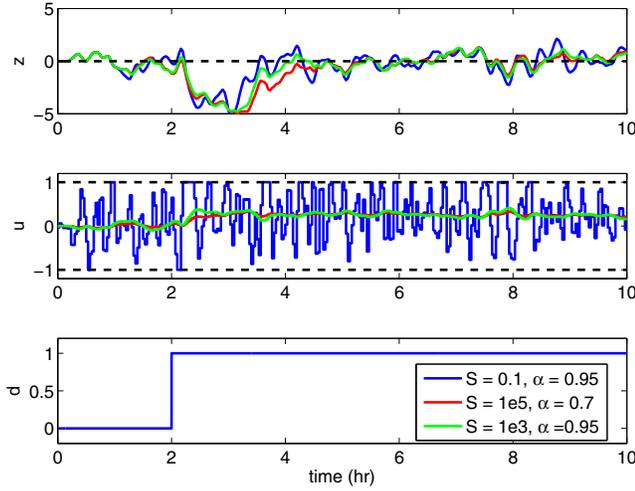
Fig. 4. Closed-loop response to a step disturbance as well as process and measurement noise for three different tunings.
