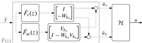
Fig. 2. The optimal  $\rho\lambda$ -FIR reconstructor
