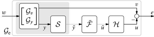
Fig. 1. System-theoretic signal reconstruction setup
