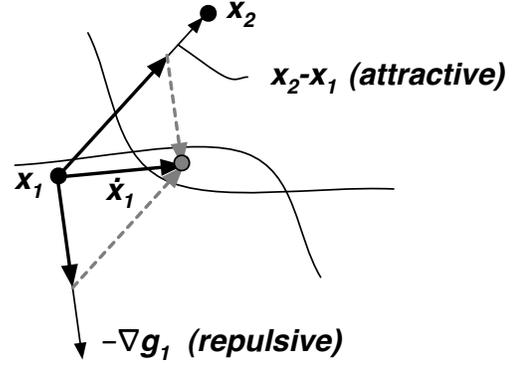
Fig. 1. Geometric illustration of the vector  $\dot{\mathbf{x}}_1$  from constrained consensus algorithm in presence of 1 neighbor
