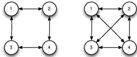
Fig. 5. Two Communication topologies for  $\mathcal{G}_1$  and  $\mathcal{G}_2$  for 4 UAVs with undirected communication links.
