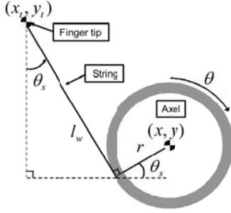
Fig. 4. Schematic figure of yo-yo model (right phase)
