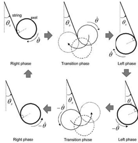
Fig. 3. Phase transition of a yo-yo system.
