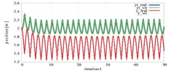
Fig. 9. The finger tip position ( $y_t$ ) and the center of gravity of yo-yo ( $y$ )
