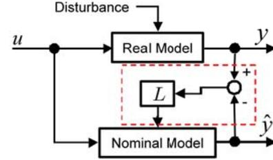
Fig. 6. Block Diagram of ILO
