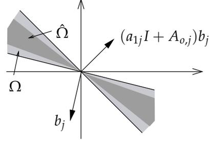
Fig. 1. Selection of the left eigenvector for  $n = 2$ . The shaded area  $\Omega$  depicts the region of all stabilizing common left eigenvectors  $\omega$ . The darker area  $\hat{\Omega}$  guarantees robust exponential stability, see Example 3.
